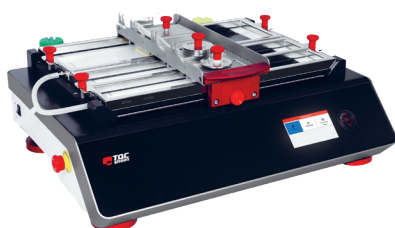
TQC Sheen Washability Tester used on the DM-40 tiles
