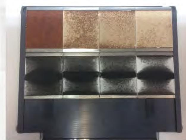
DM-tiles with inhomogenous wash results. The MACH 5 can even quantify handdish results.
